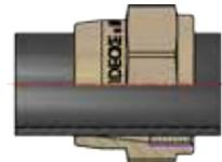
Also move the slotted squeeze ring with the cone ahead over the hose which must be cut to straight length. Make sure that the edge of the ring (labelled with the corresponding hose dimension) is flush with the hose's end.
