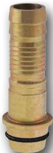
Complete Screwing Sets are extremely robust fittings for construction, tunneling and mining. A tapered stem with connecting nut is screwed with a nipple with cone. Taper and cone are sealing against each other without sealing material.
