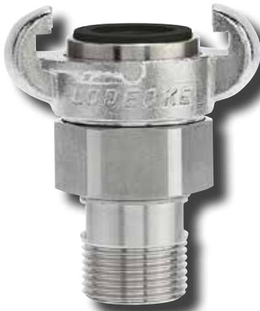
Claw Couplings are a symmetric quick coupling system with two claws each, which are connected by simultaneously applying force and rotating the two claws to be 45° apart.
