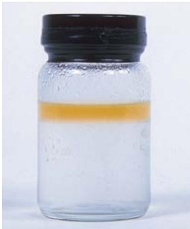
If the oil & water separates into two distinct bands, then use the ES2000 Series of static oil/water separators.
