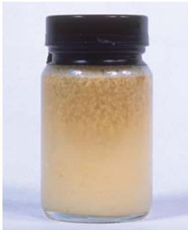
If the condensate has not separated, an emulsion separator is required.
