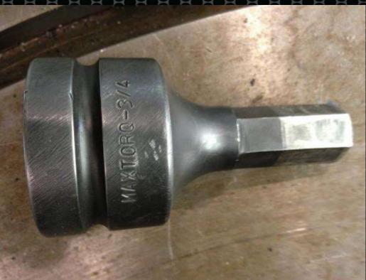
Special 19mm one piece Vascomax 1"hex drive Prevents GE from drilling out all bolts.
